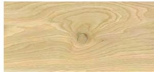
**Knots (Unsound)** — During processing, knots that dislodge/expel the core. The knot is then filled.
