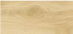
**Knots (Sound)** — During processing, knots that have still kept their original core structure.
